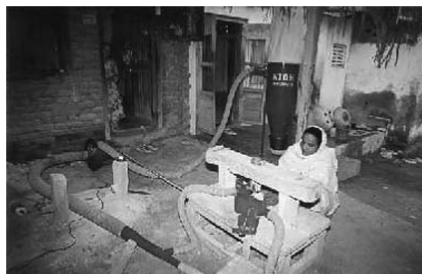
Traditional Grinding Machine with Dust Control System
